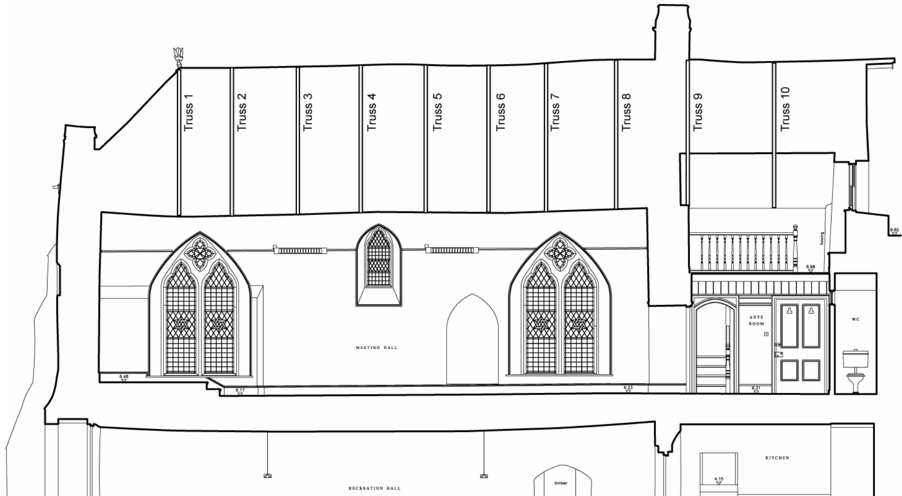
Figure 2. Longitudinal section through the Old Duchy Palace, looking east, with approximate location of the roof trusses (T1–T10) (based on a drawing by Purcell Miller Tritton LLP)
